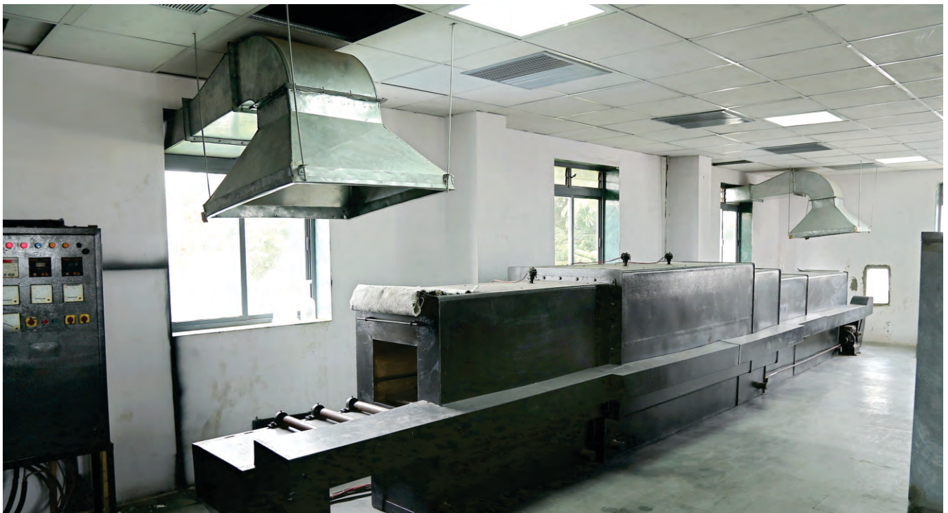
Rolling Furnace for Laboratory Items
