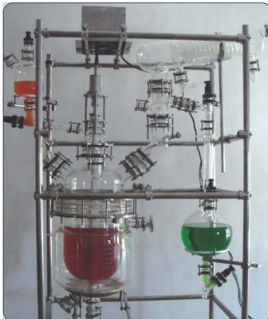
Reaction Unit with Triple Wall Jacketed Vessel
