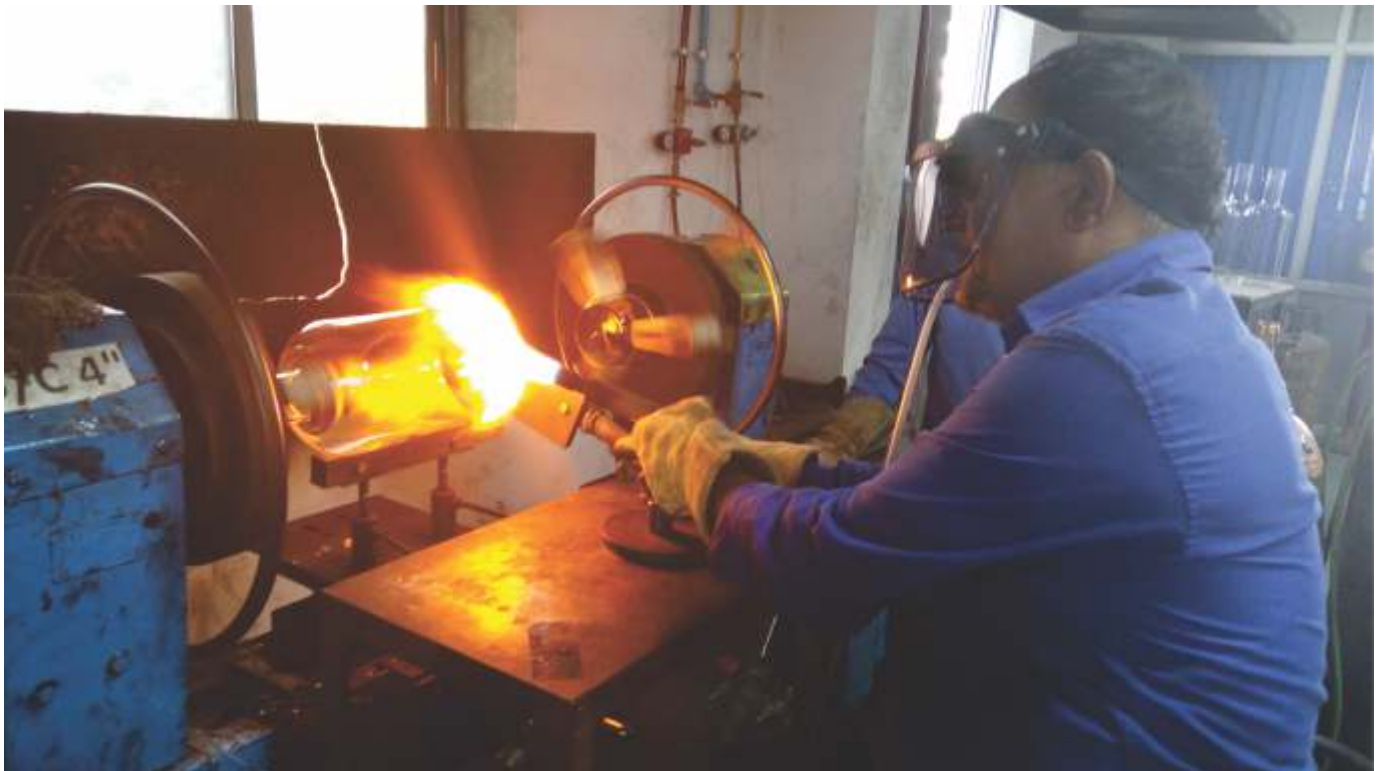
Manufacturing of solution bottle on double chuck machine by Senior Executive Chandrakant Patel
