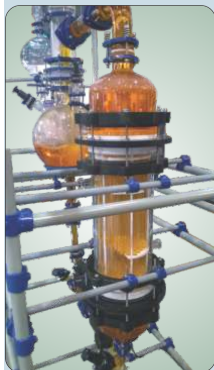
Thermo Syphon Reboiler
